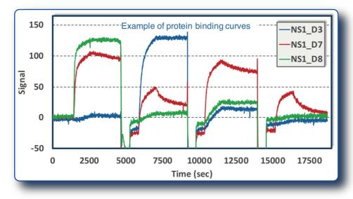
Multiplexed binding curves are extracted from the images acquired in real-time.
