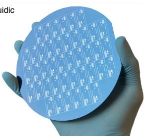
Si chips provide a large sensor area (5x7mm) and guide markings for robotic spotters for printing a microarray of ligands (\*). Reference regions and rulers enable automated image analysis and quantification (†).
