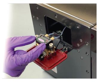
We offer low-cost and disposable sensor chips and microfluidic cartridges (patent pending) compatible with IRIS platform. Manufacturing using standard Si processing techniques provides superb quality control ensuring repeatability and scalability.
