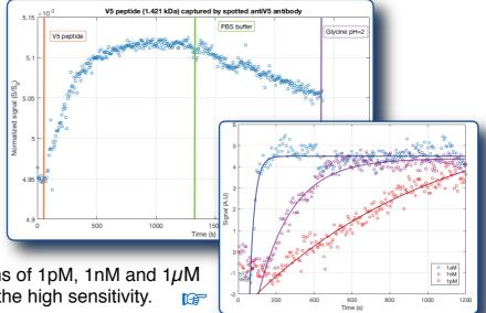
Biotin (244 Da) at analyte concentrations of 1pM, 1nM and  $1\mu$ M binding to immobilized avidin validates the high sensitivity.
